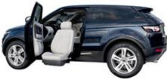
The Turney Evo, by the Swedish company Autoadapt, offers their accessible seat for use in the driver's seat. It is controlled with a handheld remote which can adjust the position of the seat, once inside the vehicle.
