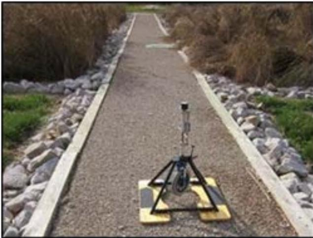
*A rotational penetrometer was used to measure the firmness and stability of the test trail segments.*
