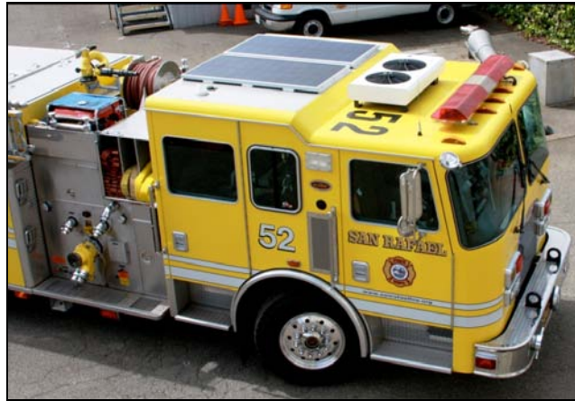
Figure 2-6: Example of PV Systems Mounted on Fire Apparatus 29 (Photo courtesy of San Rafael Fire Department)
